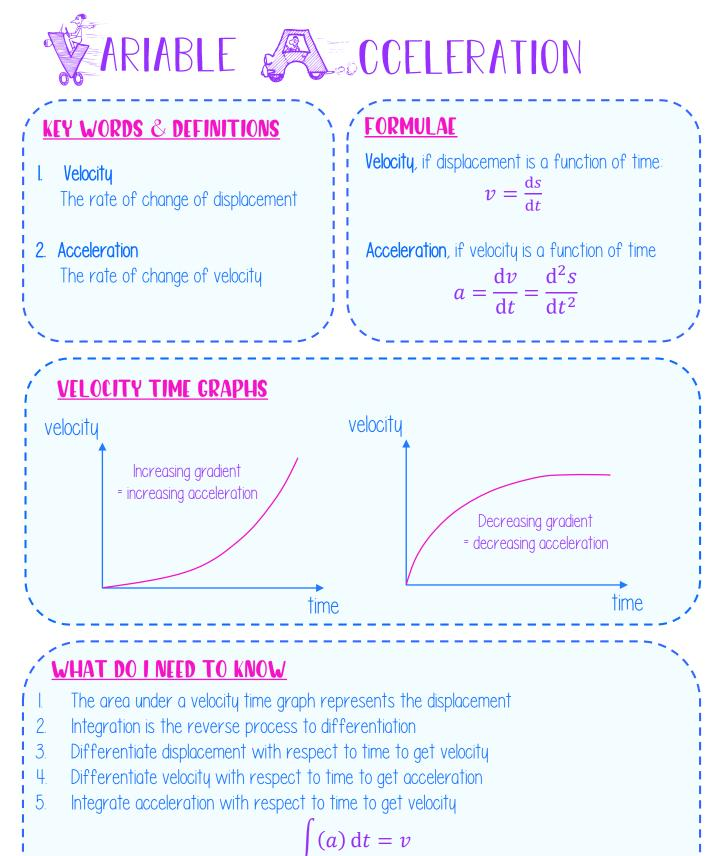
6. Integrate velocity with respect to time to get displacement
